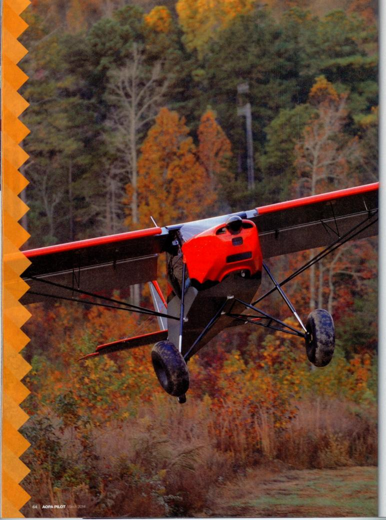
unique. There's no such thing as a power-off stall, for example. Chop the power and pull the stick all the way aft, and the SuperSTOL wing never reaches its critical angle of attack. Instead, the airplane floats down like a parachute (with a forward speed of about 42 mph and a descent rate of about 1,000 fpm). Ailerons remain effective, and so does the rudder. Landing in this configuration feels like a body slam, but the airplane seems not to mind.
